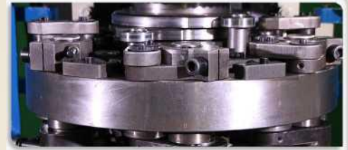
six-roller can sealing machine head is of stable and fast sealing quality.
