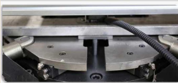
This station is all made of the high hardness, the wear-resisting import material with the function of flanging
